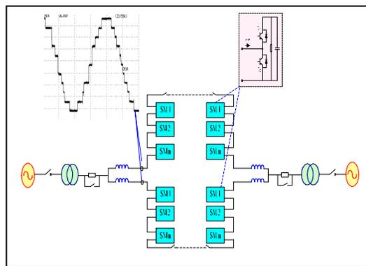
Fig.1 Typical structure of MMC-HVDC
