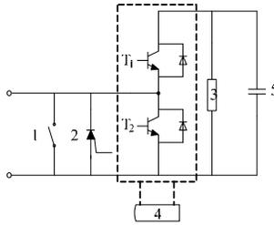
(1.bypass switch, 2. thyristor, 3.paralleled resistors, 4.SMC, 5.capacitor)
