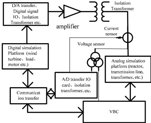
Fig.4 Interface of digital and analog subsystem
