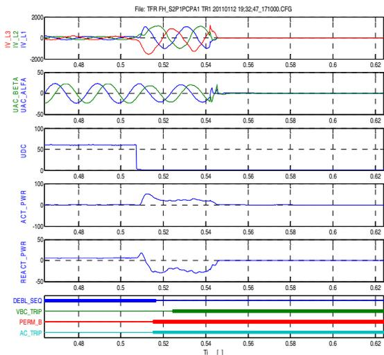
Fig.9 Waveform of protection after shortcut occurs
