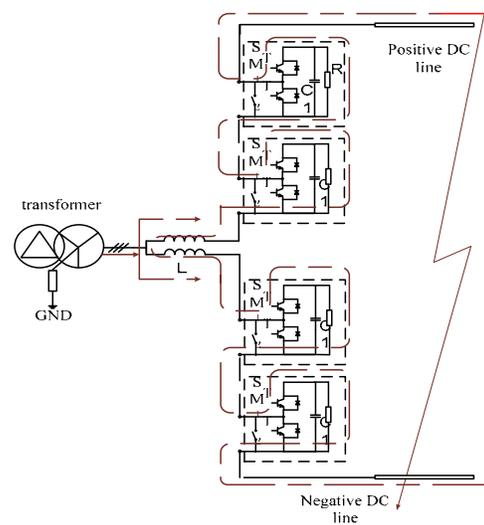
Fig.6 Current direction after dc short circuit occurred
